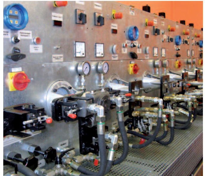
Test panel for pumps
